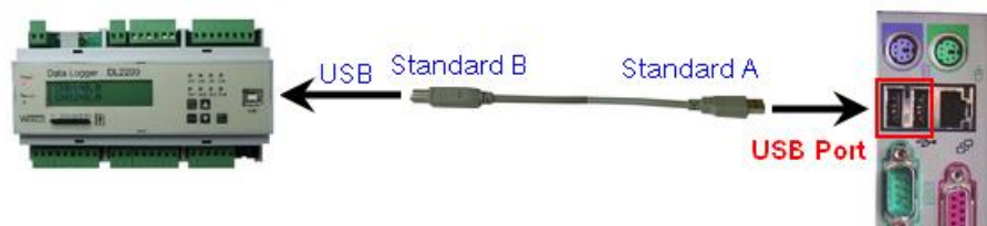
Connecting DL2200 to computer by using USB port
